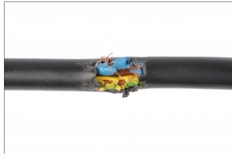
Damaged electric cable
